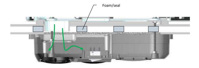
g. Connect the diffuser with the 2 plugs Faston type from the unit.
