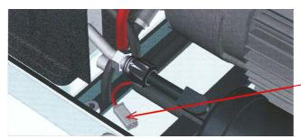
Put the cover on the unit and plug the axial fan connector.
