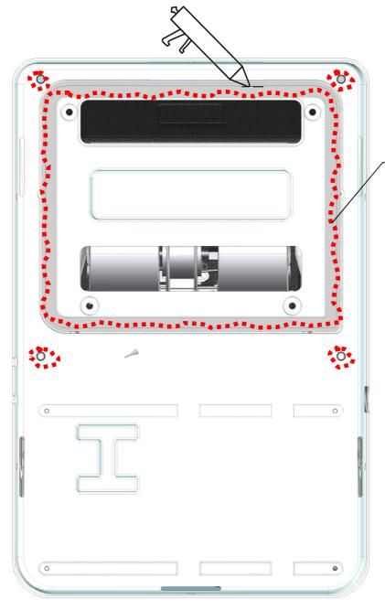
Foam 20x5mm + add the sealing strip on the foam and around the fixation points (in red).
