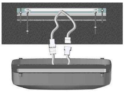
h. Put the diffuser on the 4 threaded rod and secure with 4x nuts + washers + covers
