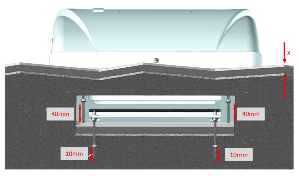
a. Cut 4 lengths of threaded rod using the following formula:
