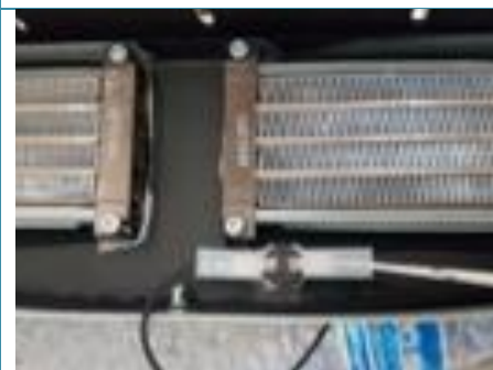
4. Connect the safety heat resistors.
