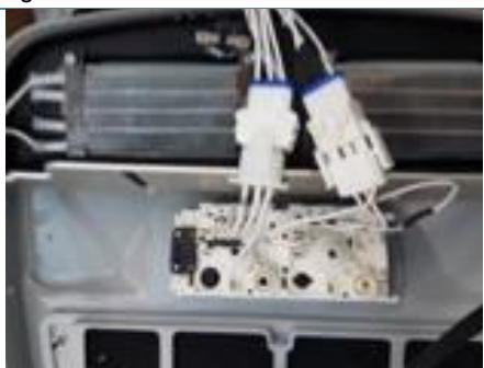
5. Connect the 3 and 6 way connectors on the control panel.
