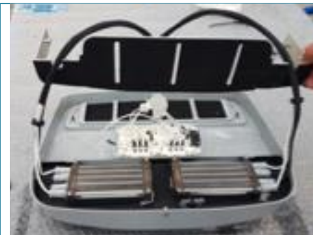
1. Feed the power of the resistor on each side of the mouting plate into the holes.
