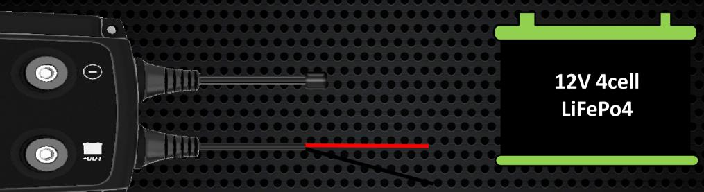
For Lithium battery selection the BLACK wire must be connected to a constant live feed +30
