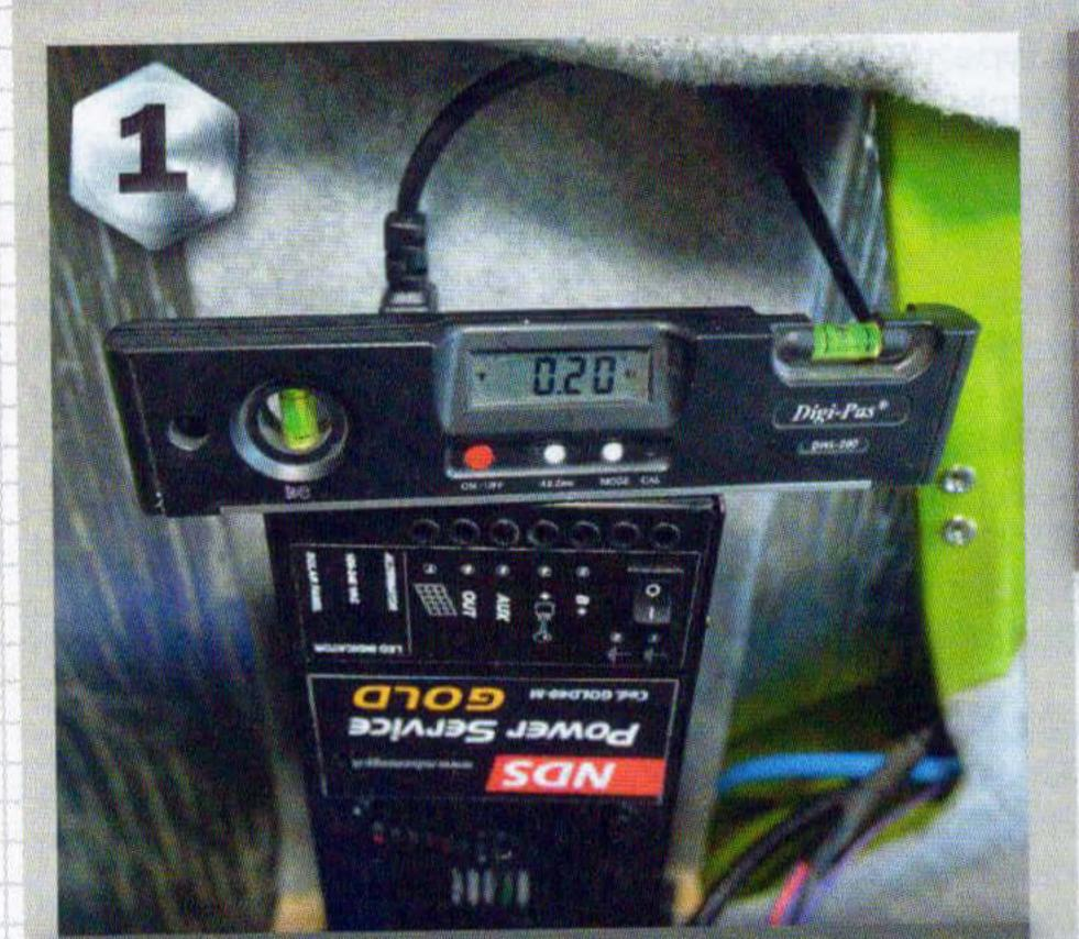
1 The first step is to mount the NDS Power Service Gold 40-M control box; this will determine the length of all the wiring. The steel case has four feet that simply need to be screwed onto a panel (a custom-made one, here)
