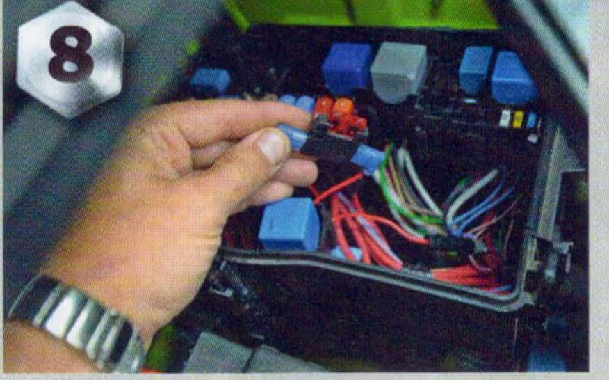
reattached, the wiring was checked and all the fuses attached under the bonnet. The LED flashes to indicate the source of power (the solar panel in this case) and the number of flashes indicates the charge programme it is in. Again, this is all explained in the
