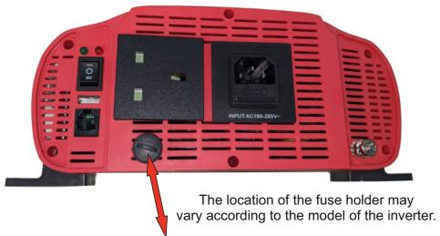
This inverter is fitted with a fuse-holder, mounted on the front panel of the unit. Inside the small plastic bag in the box, is a 15 Amp glass fuse. When the fuse is in place, the inverter **must** be connected to a dedicated RCD\* (residual current device) which protects the output of the inverter. An RCD should be used if the inverter is to be connected to the 230V sockets of the vehicle.
