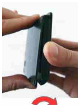
B) Lift the lower part of the display frame.
