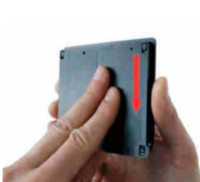
A) Slide the display's frame upwards upwards away from the back plate.
