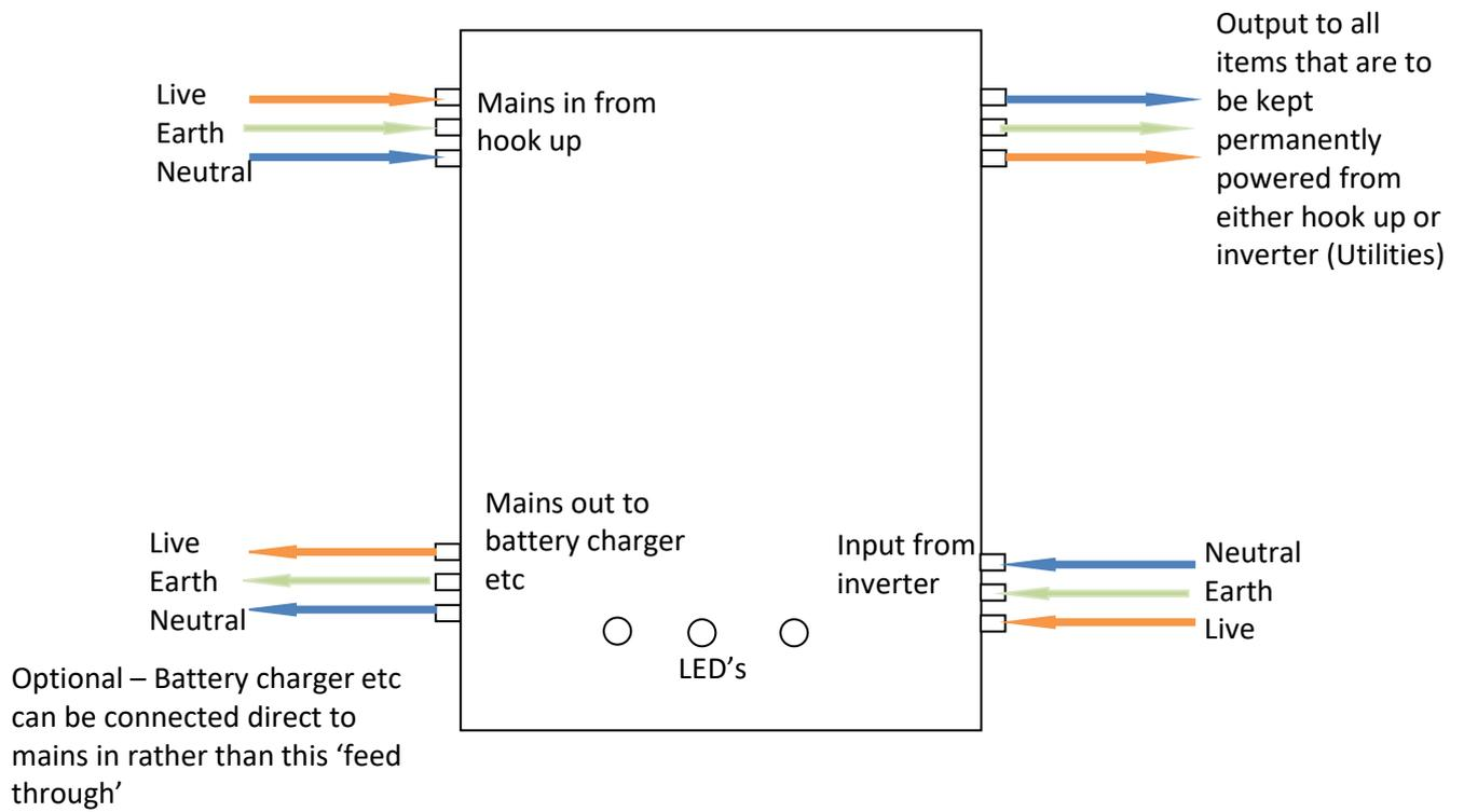
Observe mains wiring polarity
