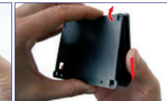
a) make the display frame slide upwards with respect to the cover behind
