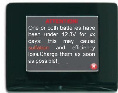
If the device is set on the "power saving" mode, this warning will be displayed upon reactivation (by just tapping the display, or by reactivating a charging source, etc.).
