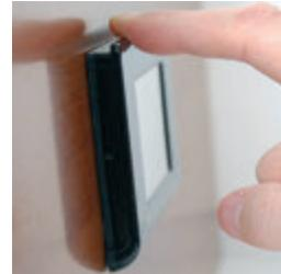
a) insert the plugs on the top of the display frame in the housings of the cover behind while keeping the lower part of the display frame with respect to the cover;
