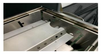
4: Locate flame diffuser shield into allocated slots on both sides
