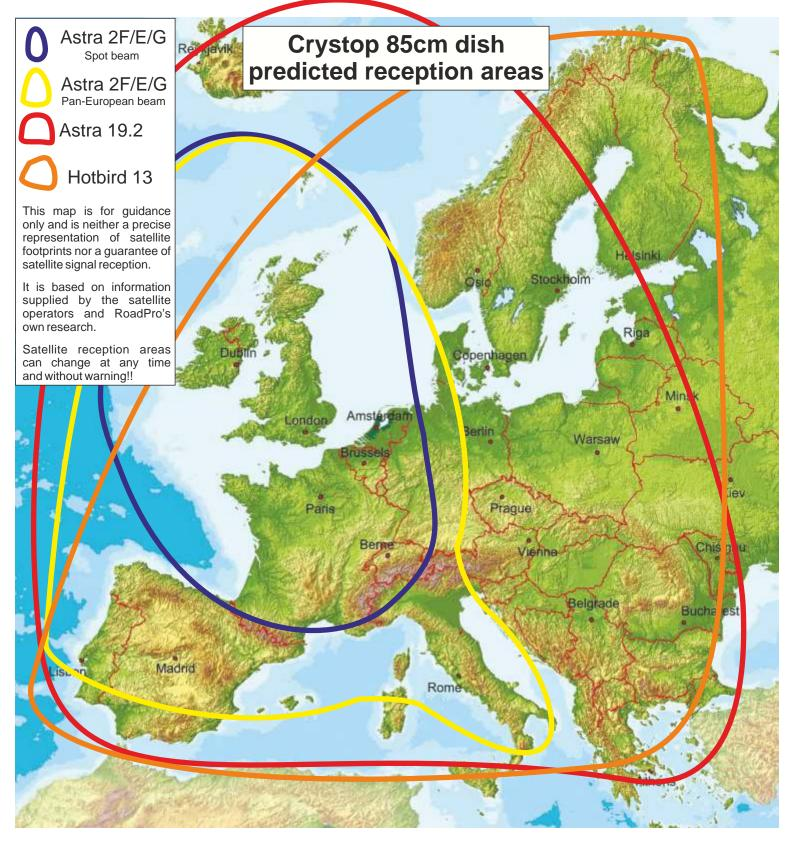
ASTRA 2E / 2F / 2G UK spot beam: All BBC, ITV, Channel 4 and Five TV channels as well as BBC radio stations are transmitted from Astra 2E and 2F.
