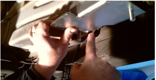
In rare cases it may be necessary to grind, for the correct rotation of the highjack
