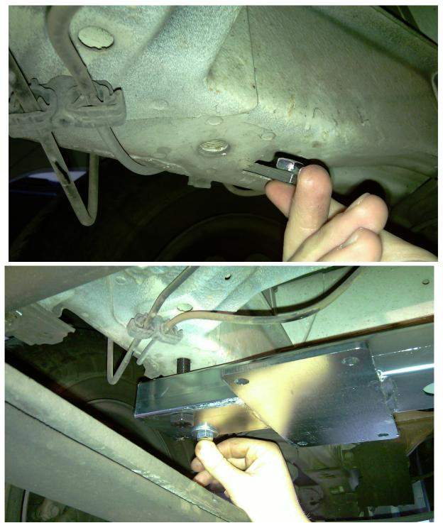
Insert and position the sealing plate (plate with **ONE HOLE**) then fix with the bolts (10x70 and 14x70).
