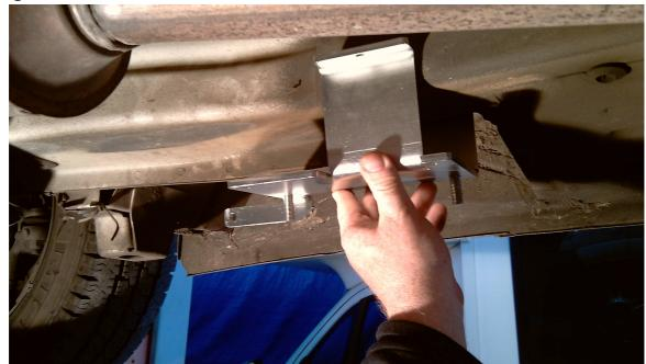
Put the adapter most rear possible, if necessary remove any sealing material for a perferct adherence, use a bottle jack to stop the bracket in the correct position and make the 8mm side hole then fix with the bolt.
