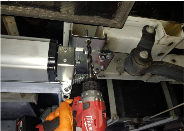
Drill a 13mm hole through the hole in the adapter.
