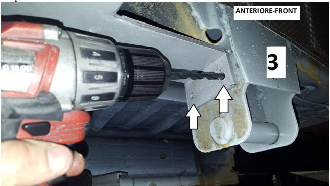
Push the adapter on the frame then drill two 10mm hole and fixs with the bolts supplied.
