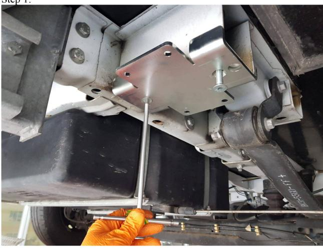
Put the adapter in the point illustrated (rear the rear axle), insert the special plates and fix the adapter with the M10 bolts supplied
