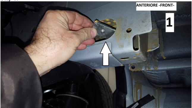
Insert the special plate throw the hole present on the frame
