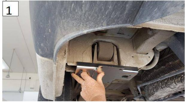
Put the adapter in the point illustrated, the rear support of the crossbow suspension
