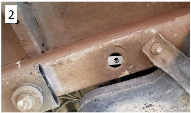
Step 1: Insert the special plate in the hole present on the frame, put the adapter and push frontly.
