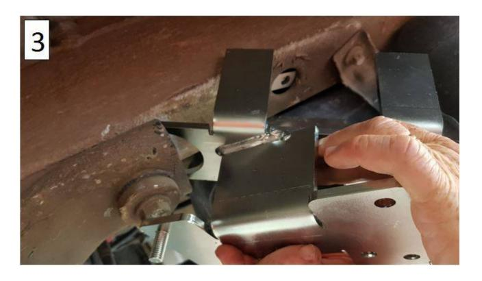
Step 2: Then fix the adapter with the bolt M10 supplied.
