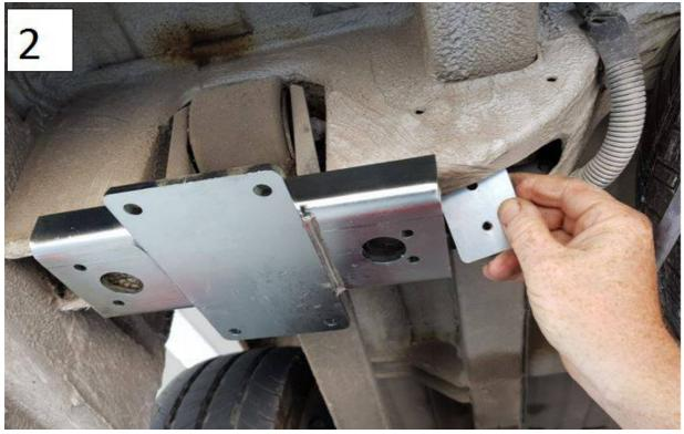
Insert the special plates and fix the adapter with the M8 bolts supplied
