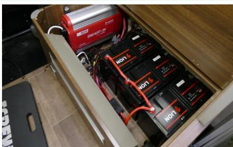
In this motorhome installation, 300Ah of NDS LiFePO4 batteries with an NDS 2kW inverter will enable the use of the air-conditioning as well as the coffee maker!
