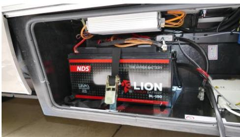
A lithium battery will usually fit in the same place as the lead-acid battery it's replacing. Even under one of the front seats is possible as there are lithium batteries available which are almost exactly the same size as standard lead-acid models.
