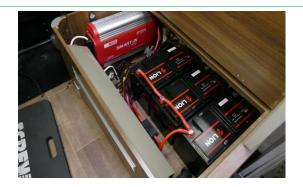
In this motorhome installation, 300Ah of NDS LiFePO4 batteries with an NDS 2kW inverter will enable the use of the air-conditioning as well as the coffee maker!
