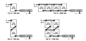
Any battery current should flow over the smart shunt. Therefore, it is to be installed directly near the battery (batteries). Correct calculation of the actual battery capacity is only possible, if all currents are detected correctly by the smart shunt.
