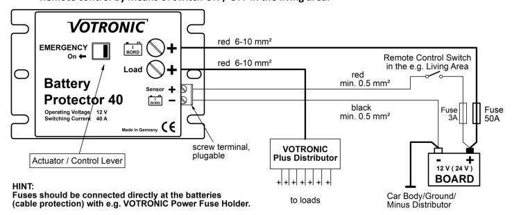
This type of switching allows an effective remote control of the unit by means of a switch being located in the living area. Since the load of the switch is very low (0.002 A), an execution as microswitch is sufficient.
