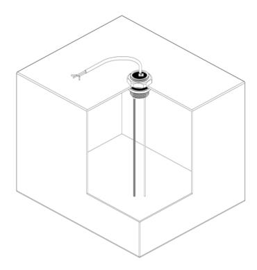
For remote level measurement, the **tank electrode** is installed directly at the tank. It is suitable for:
