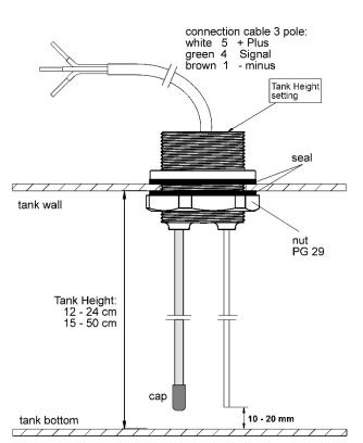
After that, the two stick probes must be cut to identical length (metal saw, strong side cutter, bolt cutter).
