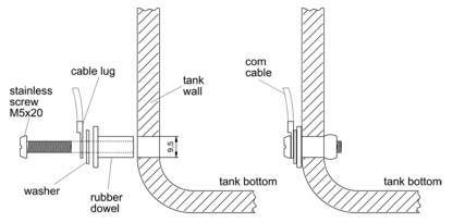
The conductor establishes the contact to the water.
