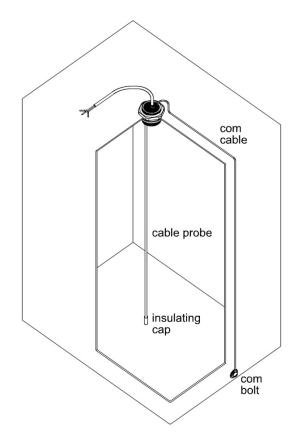
For remote level measurement the **tank electrode K-FL** is installed directly at the tank. It is suitable for:
