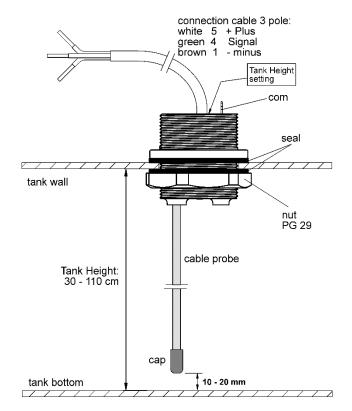
After that, straighten the cable probe, cut it to length and push the insulating cap on the end of the probe.
