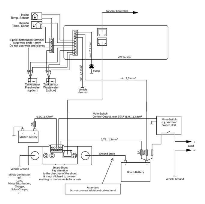
All terminals are designed in such a way, that end-type terminals are not required. The 9-pole terminal at the display panel is a plug-in terminal, which can be removed for installation. The cable cross-sections can be drawn from the plan. Since fuses serve as cable protection, they must be positioned as close as possible to the battery.
