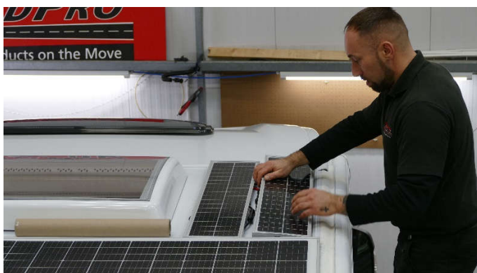
Damian installs the two 25 Watt panels.
